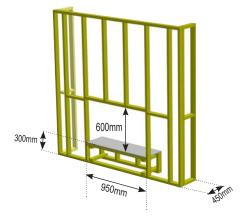
The frame and plaster cutout dimensions as shown above should be cut as accurately as possible to ensure adequate coverage by the appliance fascia. Illusion can supply fabricated full metal frames to simplify the installation and reduce costs.
